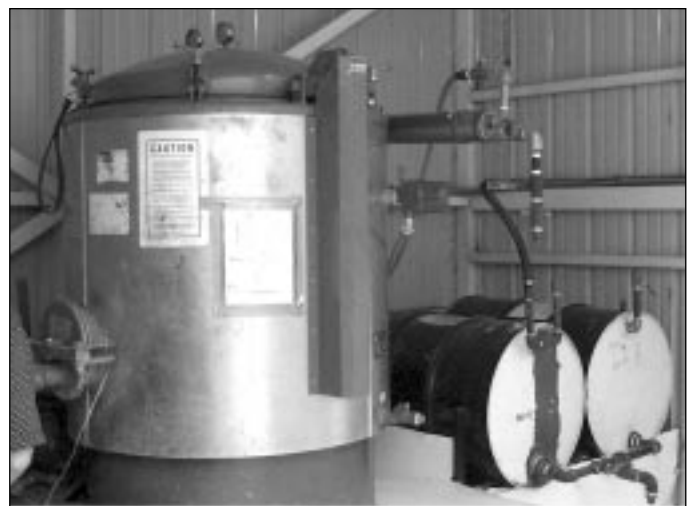
Acetone recycling unit controls temperature accurately for efficient distillation.
